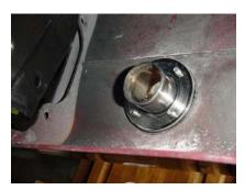
6. Install the inner flange shaped Nomex onto the outer flange tube. Install the inner flange onto the outer flange tube. Secure the assembly by tightening the (4) M6 x 1.0 BHCS (5mm hex key).
