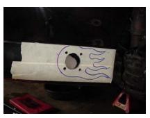
2. When you are positive on the location, drill a large hole through the bumper in the center of the small circle (1 ½" dia.) you traced. If you do not have a large drill, you can use a smaller size and make it larger with a die grinder or rotary tool (a stone wheel works best). Slowly increase the size until the Front Wastegate Dump just fits.
