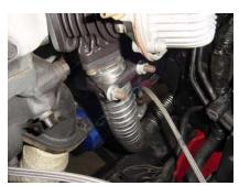
7. Remove your 1 ½" dia. wastegate outlet tube and cut it off at the best location to fit the stainless steel flex tubing. Test fit the flex tubing to determine the proper length. DO NOT cut the tubing too short, allow for slack so the tubing does not put the bumper in a bind. Attach the flex tubing to your outlet tube with the supplied 1 ½" exhaust clamp (1/2" or 13mm wrench).
