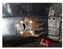
5. Install the outer flange shaped Nomex onto the outer flange. Install the outer flange into the hole you've made. Verify that you have the correct position and orientation.
