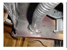
8. Install the stainless steel flex tubing to the end of the outer flange tube with the supplied 1 ½" exhaust clamp (1/2" or 13mm wrench).
