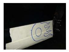
1. Determine the location to install your Jay Racing Front Wastegate Dump. Be sure there is clearance behind the bumper. Mask the area with masking tape. Use the Nomex piece that matches the outer flange as a template and trace it in the determined location. STOP! View from multiple angles and be positive that this is where you want to install your Front Wastegate Dump.
