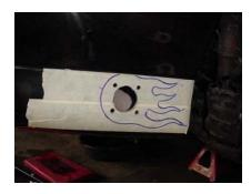
3. Place the Front Wastegate Dump flange into the hole you've made. Rotate the flange until it is the best looking orientation (typically this is when the 4 holes are parallel to the ground with the vehicle at ride height). Mark the holes with a marker, remove the flange, and drill the holes with a ½" drill bit.
